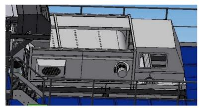
mechanical impulses if moved through an alternating magnetic field. Making use of this principle the ECS is able to sort e.g. high-purity aluminum fractions or other metals out of a material stream.
