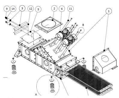
The LSM can be equipped with three stacked screen inserts resulting in four screen cuts. A wide range of different screen inserts are available.
